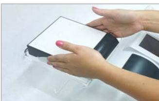
Position the scales stand behind the franking system and place the scales on to it.
