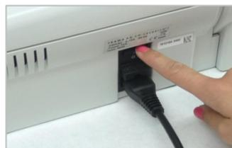
Plug power cable in to mains. Switch the franking system on.
