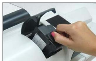
Insert the new Ink-Jet Cassette by pinching the grips of the new cassette and pushing it in to the franking machine.
