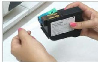
Remove the two protector strips of the new Ink-Jet Cassette being careful not to touch the gold coloured contact points.
