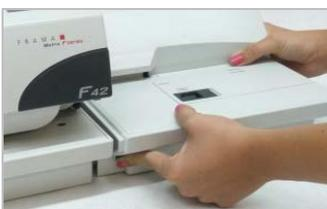
Press the release button to mount the feeder to the franking system.
