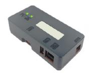
The F-Link 2 is successfully setup once you see  $\ensuremath{\text{\bf both}}$  green lights on
