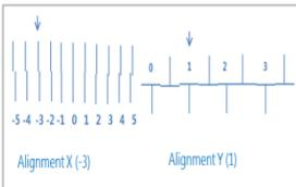
The Test Print shows current settings. The arrows should point to where the lines appear straightest.
