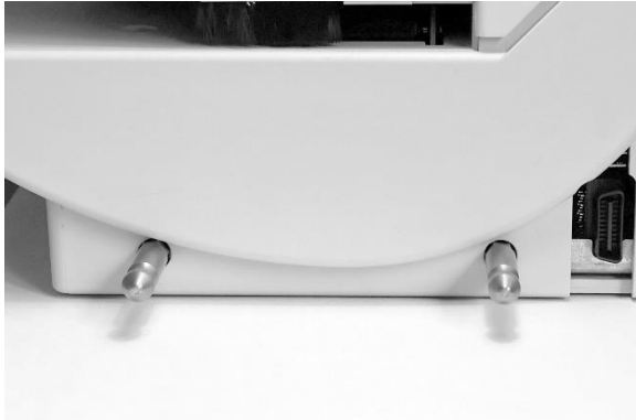
Figure 1: Matrix franking system with connecting pins
