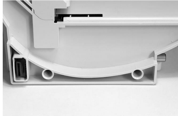
Figure 2: Automatic feeder with guide holes
