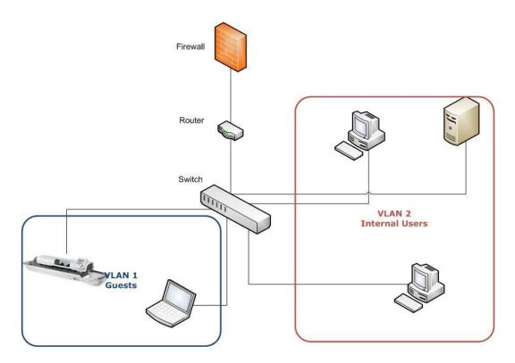
As shown in the diagram above, allocating a network segment for the Mailing System assures that network resources are shielded from possible intrusion by malicious software or users.
