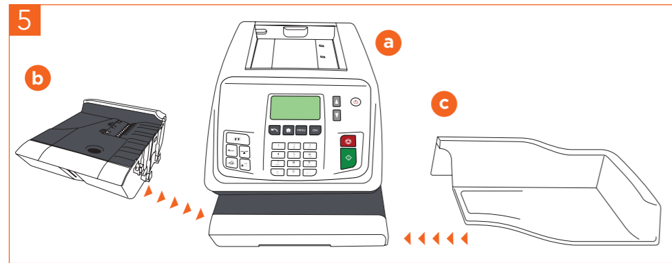
5 Lift machine slightly on the left hand side and align the hooks to attach the Feed Table (b) - align the catch tray to the right hand side of the machine (c).
