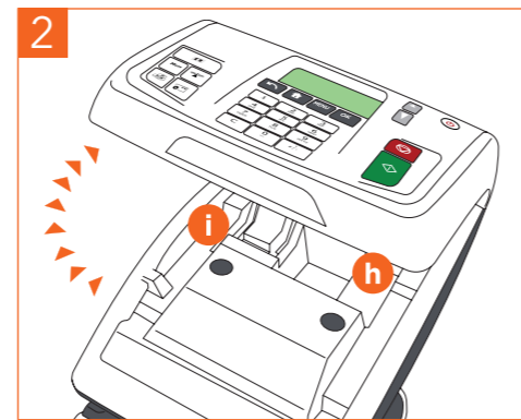
2 Lift the cover of the machine to reveal the Ink Cartridge (h) and Meter (i) locations.
