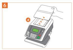
Lower weighing platform release panel at the back of the machine. Place weighing platform (d) on top of the machine and slide forward to lock. Lift panel to secure and clip cable into place.
