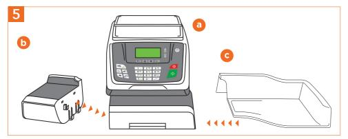
Lift machine slightly on the left hand side and align the hooks to attach the feeding table (b) – align the catch tray (c) to the right hand side of the machine.
