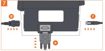
Connect the weighing platform connector (e) into the COM PORT on the back of the machine. Then connect the LAN cable (f) and power cable (g) to each side of the machine.
