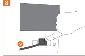
Turn on the machine using the switch behind the power cable (g) and follow the steps on screen.
