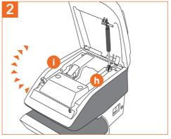
Lift the cover of the machine to reveal the ink cartridge (h) and meter (i) bays.
