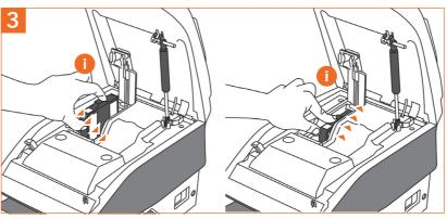
Open the cover. Place the meter (i) into the meter compartment and push backwards until it fits securely into position. Close the cover.
