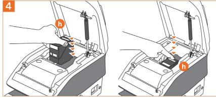
Insert the ink cartridge (h) at an angle into the machine with the 'TOP' and 'LOCK' stickers facing upwards. Push the ink cartridge (h) towards the back of the machine until you hear a 'click' - close the cover of the machine.
