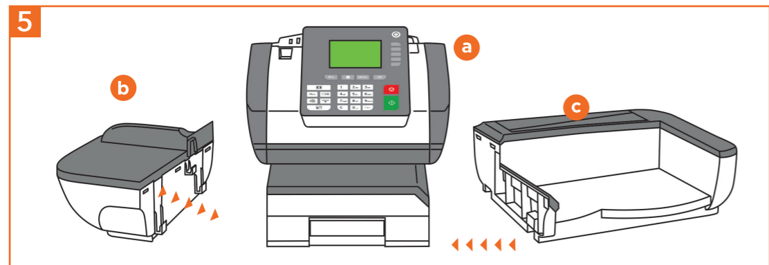
5 Lift machine slightly on the left hand side and align the hooks to attach the feeding table (b) - attach the catch tray (c) to the right hand side of the machine.
