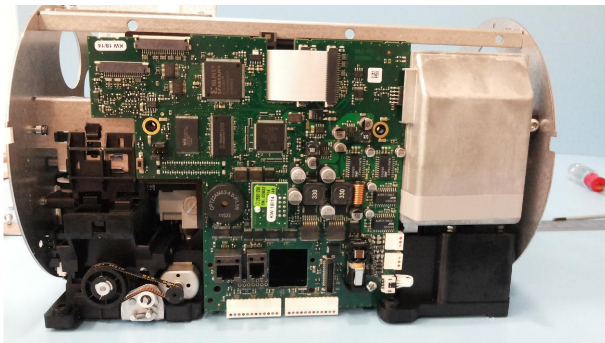
Figure 9 – Main board view
