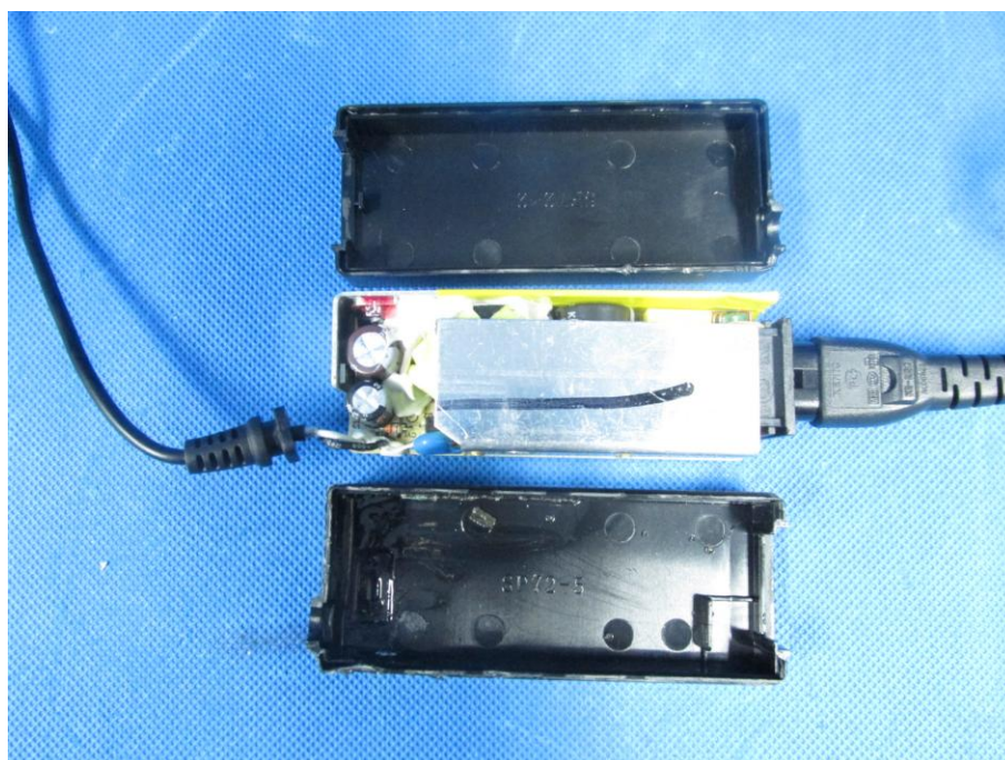
Figure 13 – Internal view 1 of external power supply
