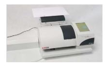
Place a letter on to the scales. Depending on the selected weighing mode put one letter (single weighing mode) or a stack of letters onto the scale platform.
