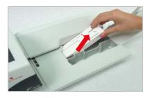
Insert the new label box. Fix the labels in to the box using your finger (see arrow in example), push it in and to the left as far as it will go.
