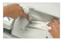
Pull the hook clamp up again and push the left end of the new label box under the hook clamp. Use your finger to fix the labels in the box.
