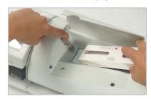
Hold the hook clamp in this position and remove the label box.
