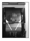
Release the grip surfaces. Push the ink jet cassette back with one finger to make sure that the locking tabs are correctly positioned and that the ink jet cassette is locked into place.
