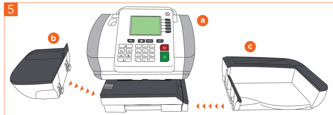
5. Lift machine slightly on the left hand side and align the hooks to attach the Feed Table (b) - attach the Catch Tray to the right hand side of the machine (c).
