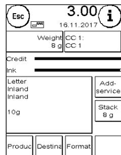
Take the next letter from the stack. The weight of the letter is displayed and the postage calculated accordingly and so on. Once you have removed the last letter from the stack, the stack weighing mode is quit after 3 seconds.
