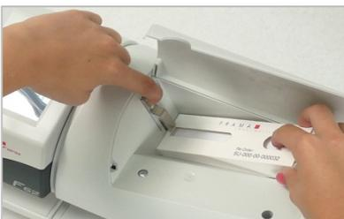
Pull the hook clamp up again and push the left end of the new label box under the hook clamp. Use your finger to fix the labels in the box.
