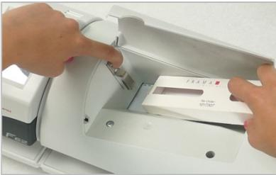
Hold the hook clamp in this position and remove the label box.
