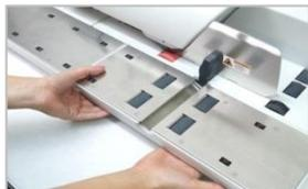
Position the tables and turn the locking lever to the left to fix in place.
