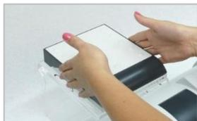
Position the scales stand behind the franking system and place the scales on to it.
